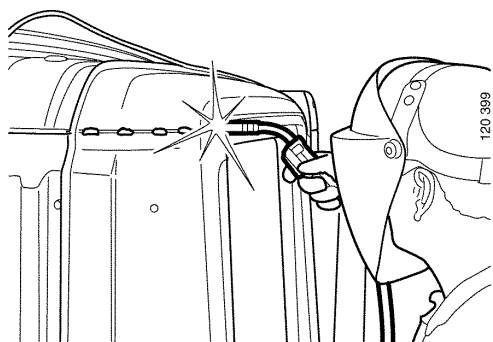
Note: Applies to the 14-cab only. Weld the roof joint from outside.
