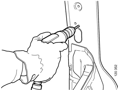
Drill away the spot-welds.
