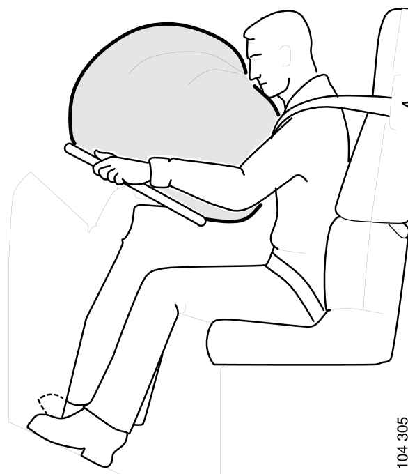
Belt pretensioner and airbag
