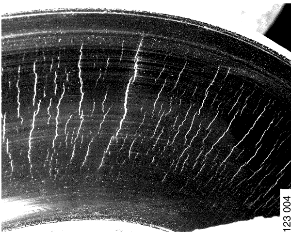
Permitted crack formation
